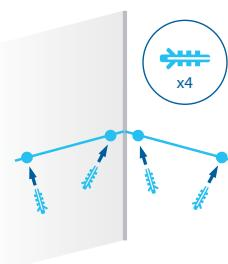
After drilling the holes, insert the wall plugs provided in the package (D).
