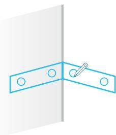
Put the paper template included in package (E) on top of the drawn lines, and mark the 4 shelf fixing holes (2 for each side of the corner) with a pencil.
