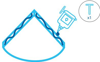
Remove the shelf and apply in the shelf slots the adhesive sealant (C) provided in the package, using, if necessary, the tube squeezer (F). In case you would fix the item in a humid environment, such as a shower box, please ensure to cover the full perimeter of the product for optimum sealing capacity.
