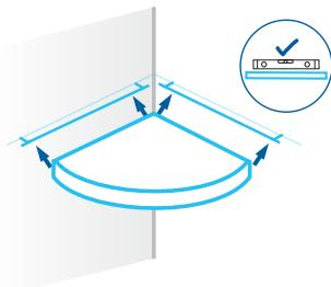
Temporary insert the shelf (B) in the steel brackets and verify if it is levelled.
