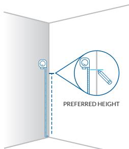
Set the height from the floor where you wish to install the shelf and mark with a pencil a small line on both walls near the corner.
