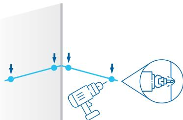
Using an 8 mm (1/3") drill bit, drill 4 holes on the 4 spots you marked.
