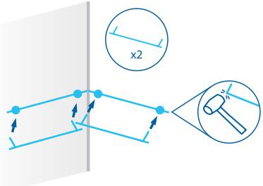
Insert the 2 steel brackets provided in the package (A) into the wall plugs, using a rubber mallet hammer if required.
