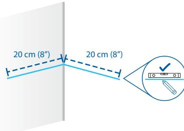
Once you have defined the desired height and position, draw a horizontal line of about 20 cm (8") long on both walls, starting from the corner. Use a level for increased accuracy.
